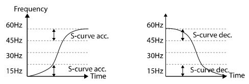
[Acceleration / deceleration S-curve pattern configuration]
