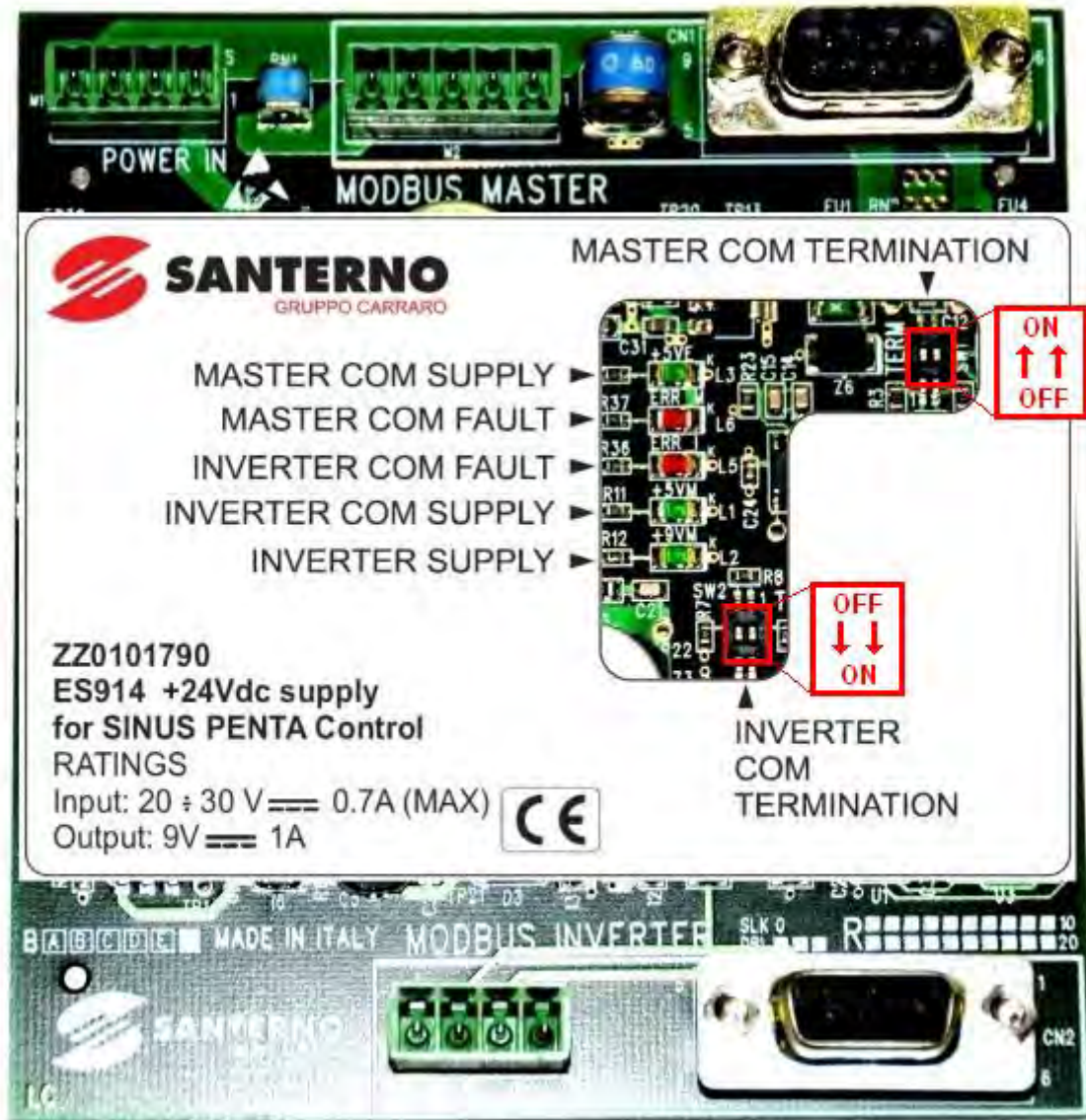
Figure 217: Position of the LEDs and DIP-switches in ES914 board
