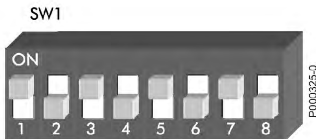
Figure 223: DIP-switch SW1 setting in three-channel mode
