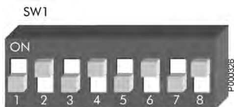
Figure 224: DIP-switch SW1 setting for five-channel mode
