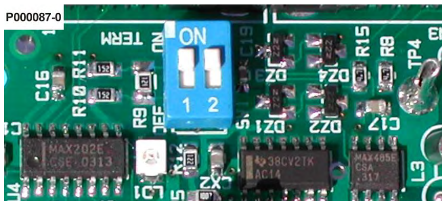
Figure 154: Configuration of terminator DIP-switch for line RS485
