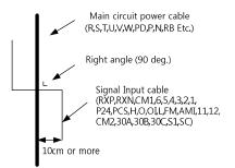
Figure 2-7 Separate of main circuit and control circuit wire
