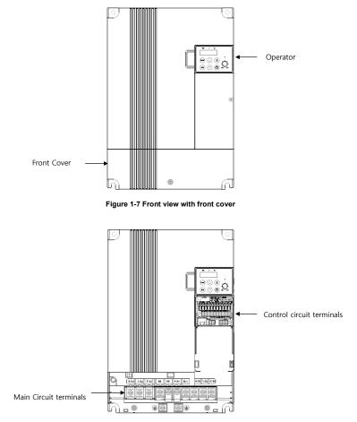
Figure 1-8 Front view without front cover
