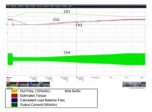
2) Put 100% step load and removed 100% load in a moment
