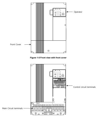
Figure 1-6 Front view without front cover
