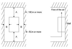
Figure 2-1 Air gap (Installation)
