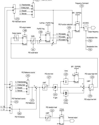
Figure 3-1: PID diagram
