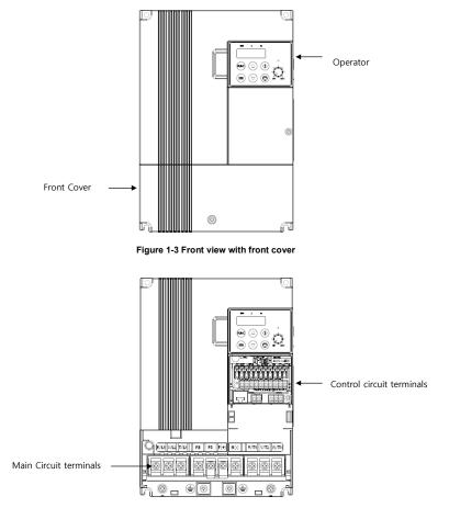
Figure 1-4 Front view without front cover
