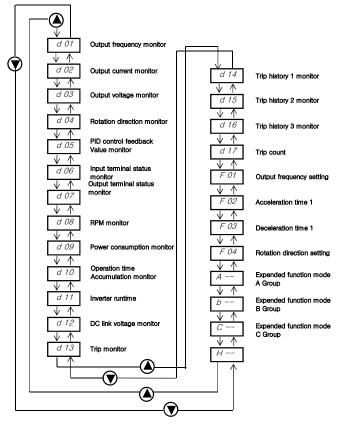
Figure 4-2 Up/Down key basic operation
