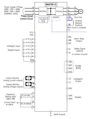
Figure 4-6 Setting diagram from the terminal
