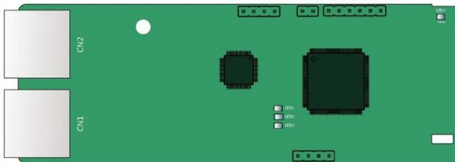
The communication port adopts standard dual RJ45 interfaces, and the two RJ45 interfaces are not distinguished from each other and can be interchangeably inserted.
