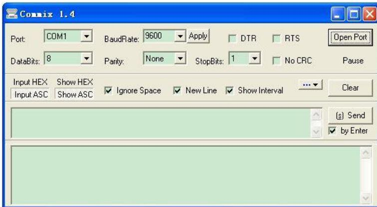
First, set the serial port to **COM1**. Then, set the baud rate consistently with P14.01. The data bits, check bits, and end bits must be set consistently with P14.02. If the RTU mode is selected, you need
