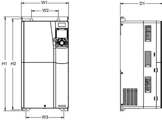
Figure C-5 045G/055P-075G/090P wall-mounting diagram
