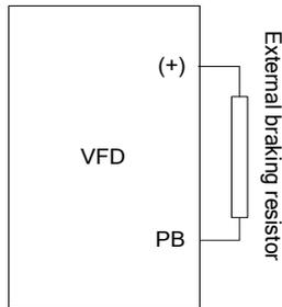
Installation of braking units:
