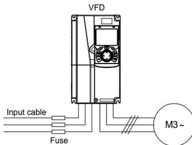
Figure 4-19 Fuse configuration
