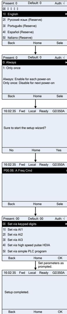
Figure 5–22 Power-up setup wizard
