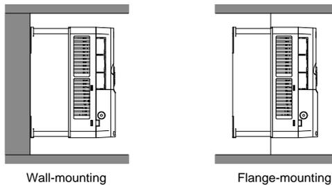
Figure 4-2 Installation mode
