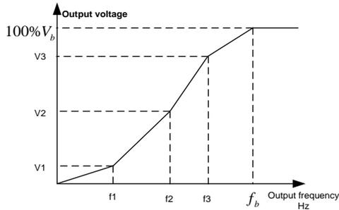
The VFD provides dedicated function codes for the space voltage control mode. You can improve the space voltage control performance by means of setting.
