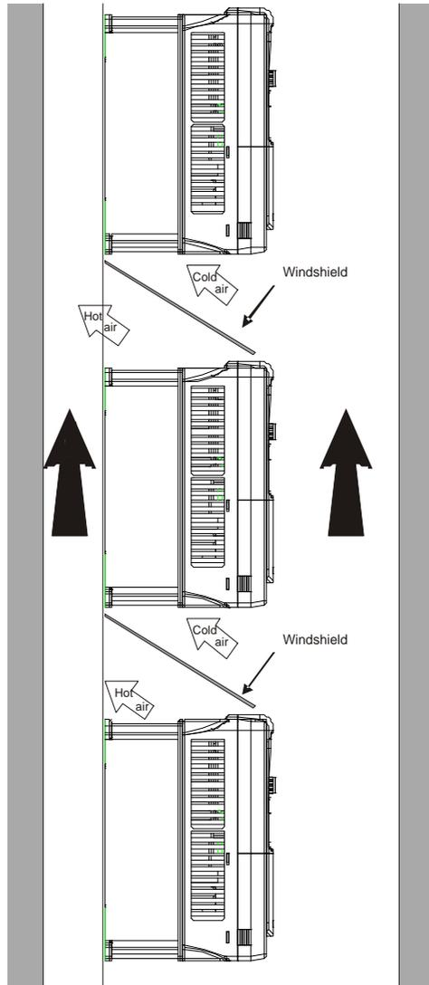
Figure 4-5 Vertical installation
