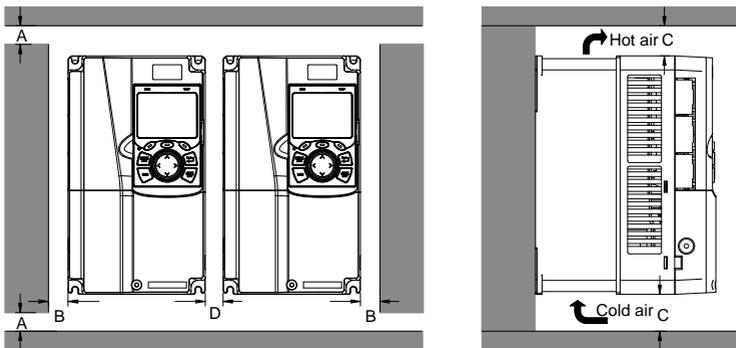
Figure 4-4 Parallel installation
