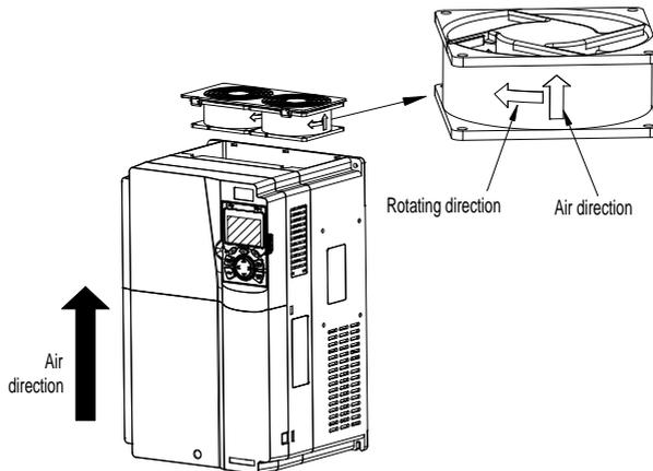
Figure 8–1 Fan maintenance for 7R5G/011P and higher models
