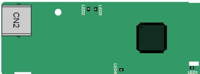
The EC-TX504 communication card adopts standard RJ45 terminals. It is used only on the upper computer that supports INVT Workshop. If you want to support the standard EtherNet/IP protocol, select the card EC-TX510.
