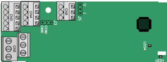
CME and COM are shorted through J3 before delivery, and J5 is the jumper for selecting the output type (voltage or current) of AO2.
