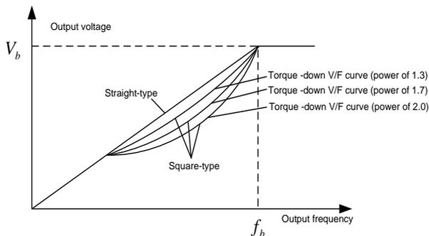
The VFD also provides multi-point V/F curves. You can change the V/F curves output by the VFD by setting the voltage and frequency of the three points in the middle. A whole curve consists of five points starting from (0Hz, 0V) and ending at (motor fundamental frequency, motor rated voltage).
