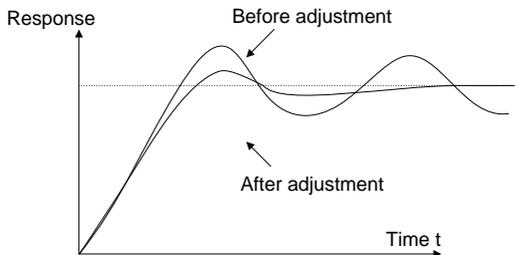
**Control short-term vibration:** If the vibration cycle is short is almost the same with the set value of derivative time (Td), it indicates derivative action is too strong, shorten the derivative time (Td) to control vibration. When derivative time (Td) is set to 0.00 (namely no derivative control), and there is no way to control vibration, decrease the proportional gain.
