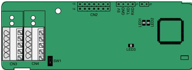
The switch SW1 is used to set the voltage class (5 V or 12 V) of the power supply of the encoder. The switch can be operated with an auxiliary tool.
