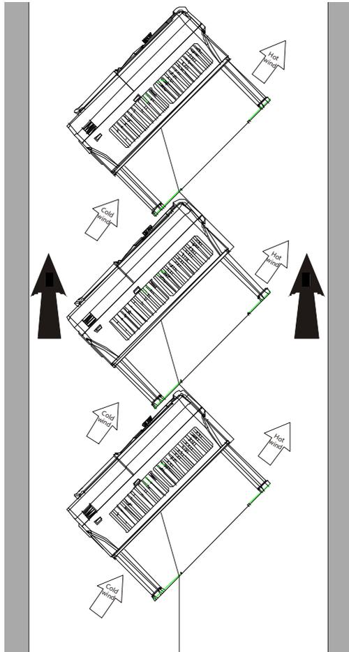
Figure 4-6 Tilted installation
