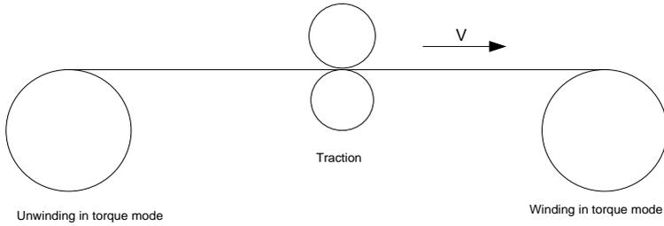
In some special situations, if the roll diameter can be counted through thickness, the following applications can be implemented:
