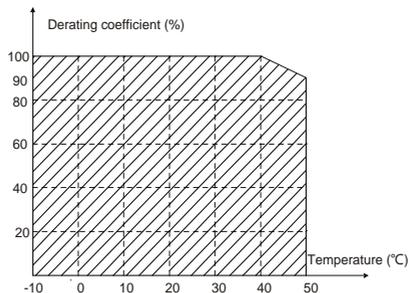
**Note:** It is not recommended to use the VFD at a temperature higher than 50°C. In case of violation, we shall bear no liability for the consequences caused.
