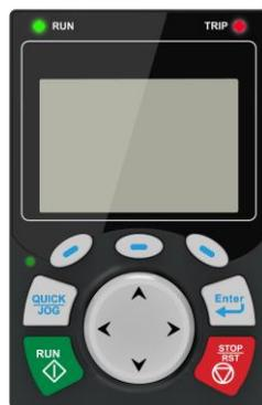
Figure 5-3 Optional LCD keypad
